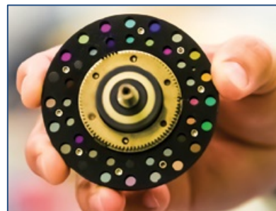
MOE Filter Wheel (Halliburton)
